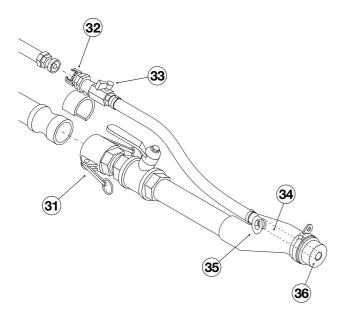
Generally speaking, with deflectors having a smaller diameter the material is sprayed with a wider pattern and vice-versa.
