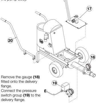
Secure the lifting handles (20).
