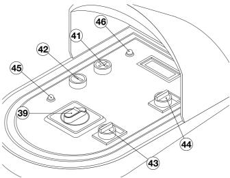
Turn the selector start/stop/reverse (40) on position  $\underline{1}$  and check that the machine is pumping normally and modify the output according to your necessity through the buttons that set the output "plus" (41) and "less" (42).
