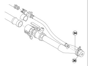
Disconnect the hoses from the mortar pump hoses and insert one cleaning sponge into the hose.
