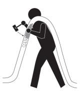
•Turn the machine on for several seconds, and make certain that the hose has been freed of the "plug": the material will flow normally from the hose. Pour some slurry into the hose before the point where the blocking occurred (gun direction), connect the hose line once again, and start over again.
