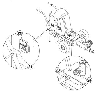
Connect the silicate feeding hose to the quick coupling (23), the other end of the hose must be connected to the vessel containing the silicate
