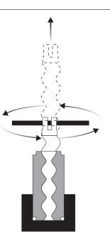
To assemble the unit, smear both the worm and the stator with vaseline (under no circumstances should you use oil or mineral grease! Such products could cause irreparable damage to the stator). Then screw the worm back into the stator. The stator must be mounted with its countersunk side facing the hopper.
