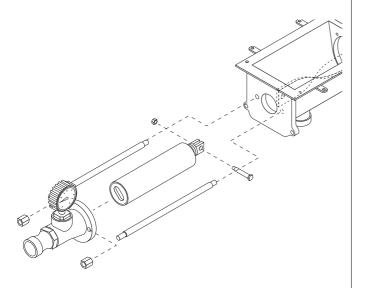
Put the group statorworm in a vice, block the stator, unscrew the rotor and remove it;
