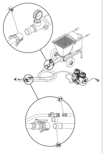
Connect the air hose to the auxiliary compressor (27) at the spray gun.
