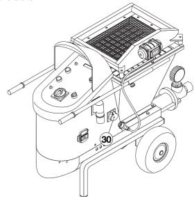
Connect the plug of the vibrating sieve to the socket (30).
