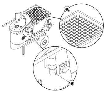
Put the cap on the hopper discharge collector and fill the hopper with water.
